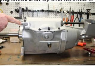
Insert Pushpin into hole of emptied plug with the red tip pointing towards you.
