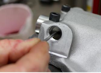
Thread Neutral Safety Switch in and tighten.
